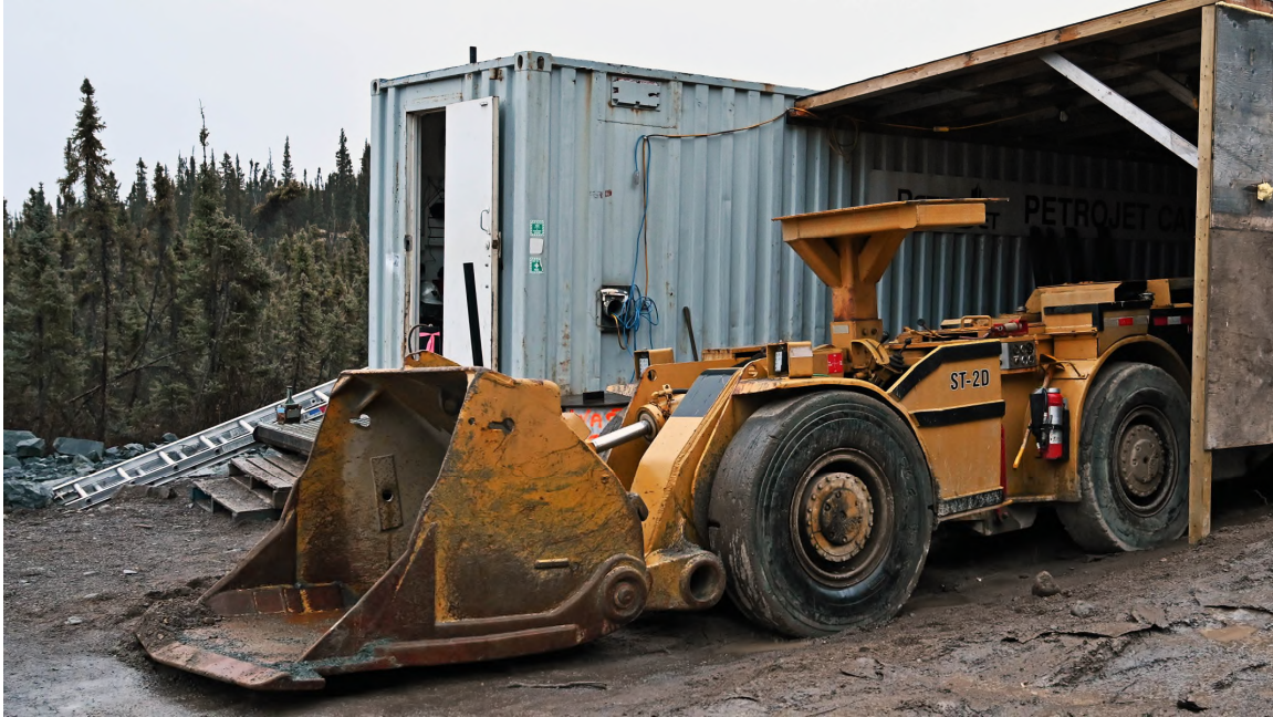
Photo 6. Two yard scooptram under cover for repairs.
