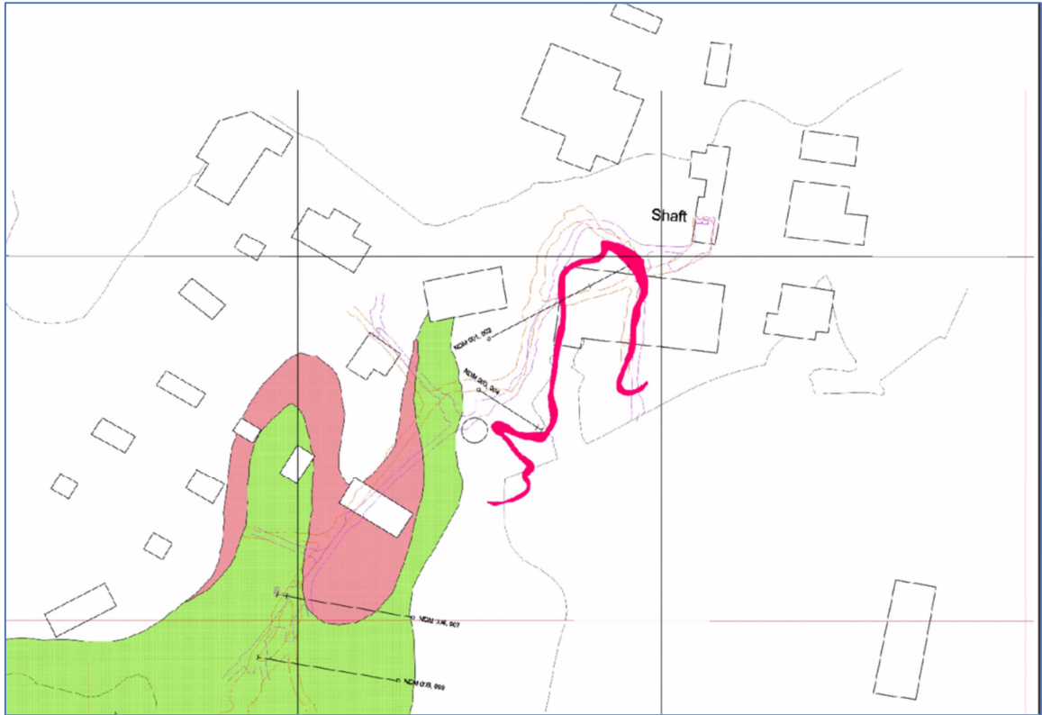
Figure 63. Plan view of the Discovery Mine with the folded quartz vein shown in red with 100 m grid.
