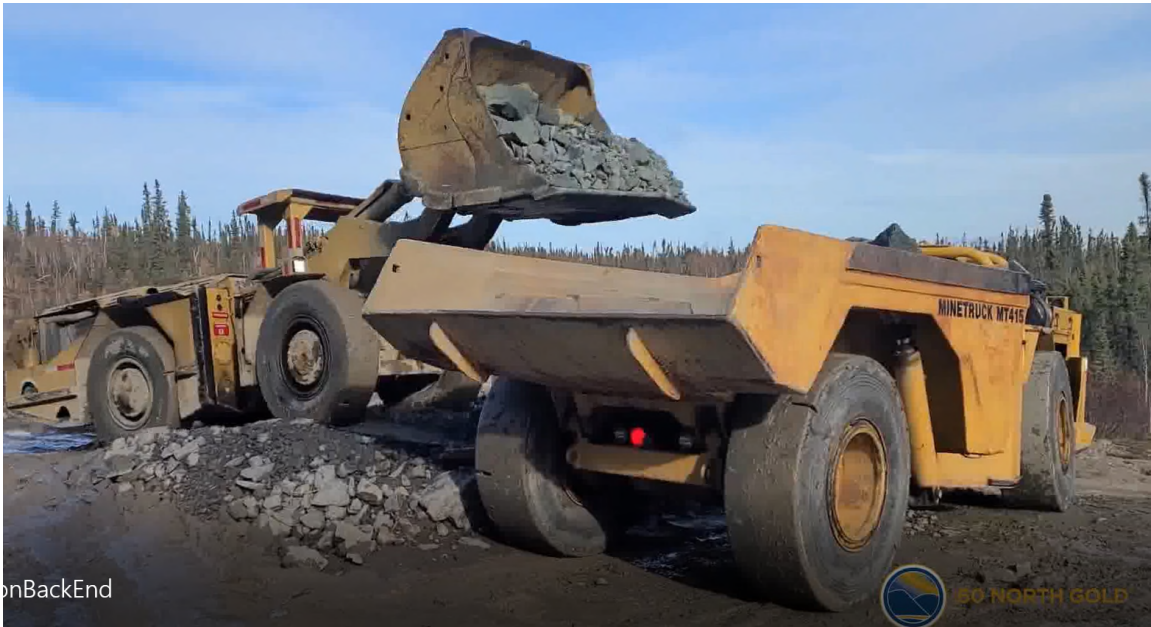
Photo 7. Scooptram loading 10 ton mine truck.
